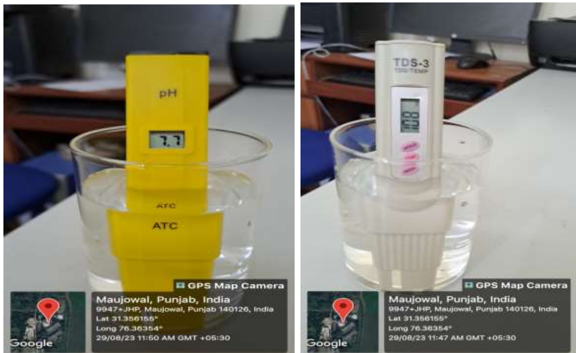
Measured pH value and TDS Value of RO filtered drinking water
